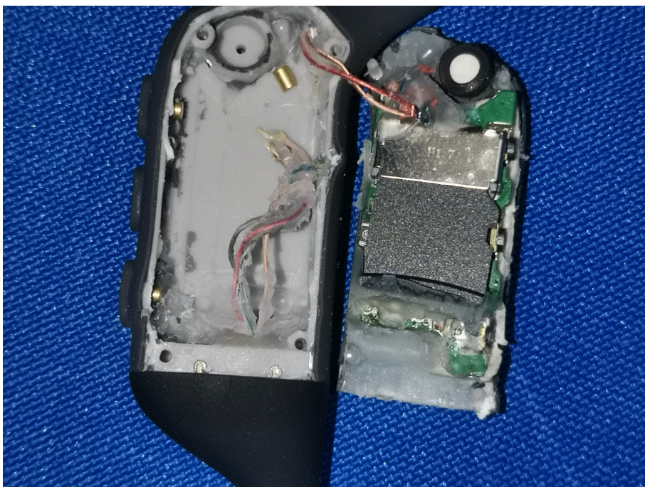
Photo 4: Test result of IPX8 test
