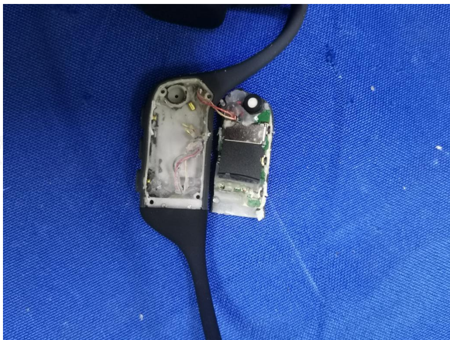
Photo 5: Test result of IPX8 test
