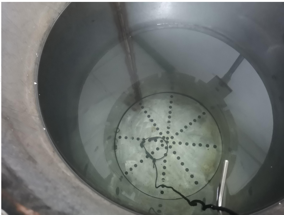
Photo 3: IPX8 test of model X16
